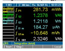
Simultaneous display of up to 6 configure able numeric values. Start/Stop conditions and positive negative direction available.
