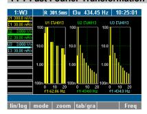
Calculation of harmonics with graphical representation. Up to 3 bar graphs are displayed at the same time.
