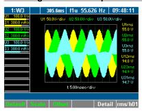
Simultaneous display of up to 3 measured values on sample level. Quick view of curve form and distortion.
